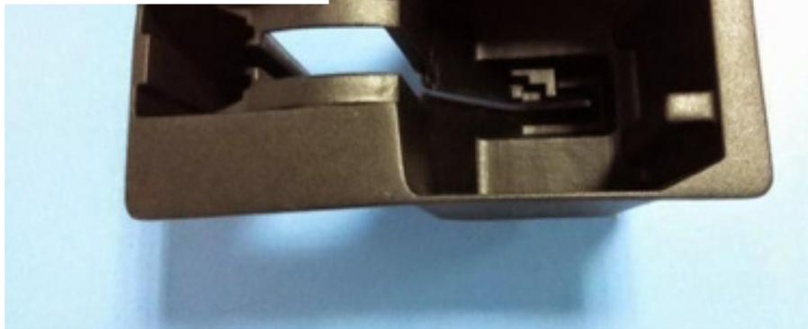
Ultra small skimming device located inside the cover of the card reader.
